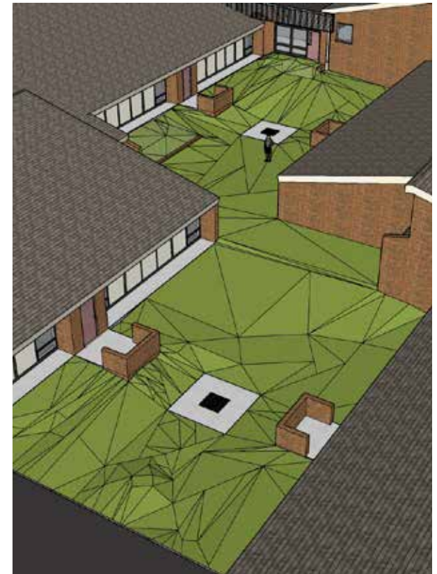
Polygonal model of terrain contours within Courtyard D, distinct faces shown
