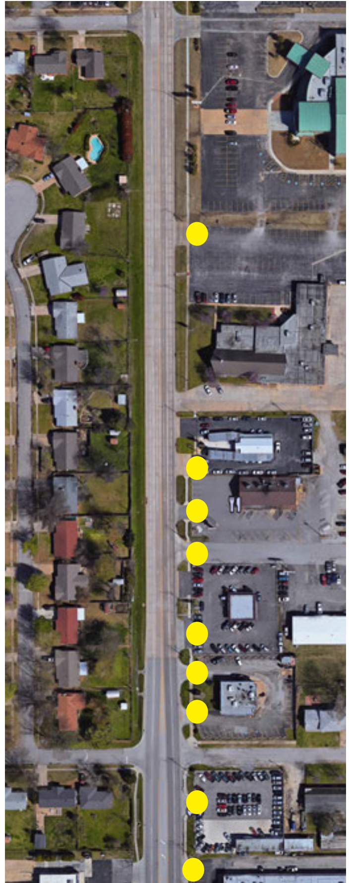
Existing Curbcuts Along Elm PI
