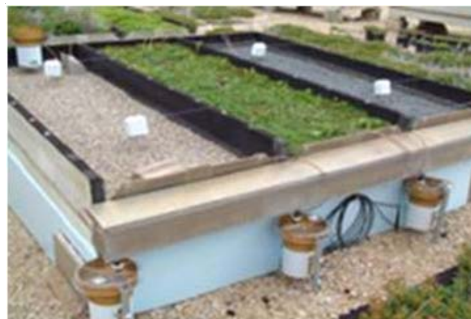
Above: 8' x 8' test platforms, featuring enclosed gutters and tipping bucket rain gauges that log data every 5 minutes.
