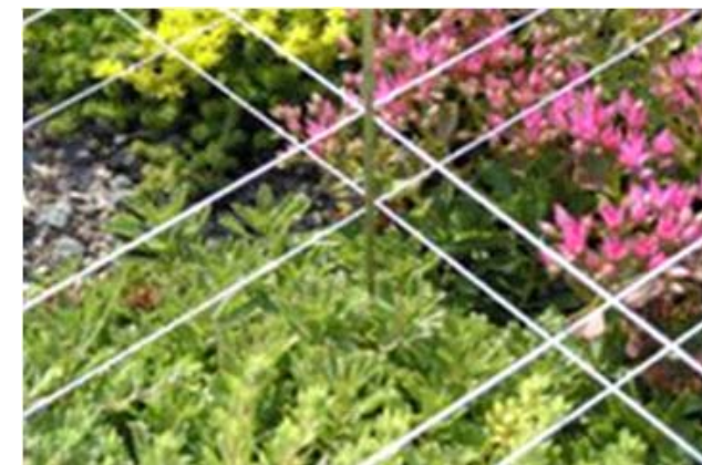
This point frame transect was constructed to measure leaf area index at three different canopy heights across test roof platforms.
