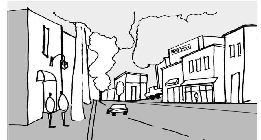
Building setback at right breaks up the continuity of the streetscape
